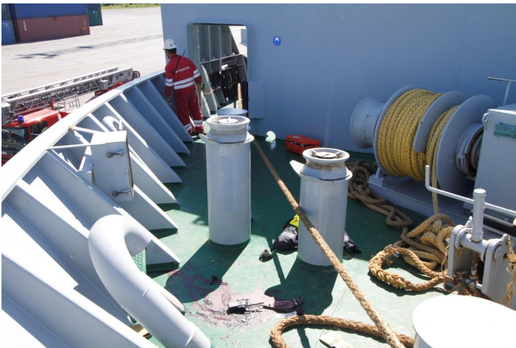
Fig. 4, Forecastle deck, opposite direction. Through the opening in the bulwark the spring line fairlead can be seen. To the right the wind lass drum with the remaining's of the parted spring line. It has not been established which of the pedestal leads where used. (Photo from the Police)
