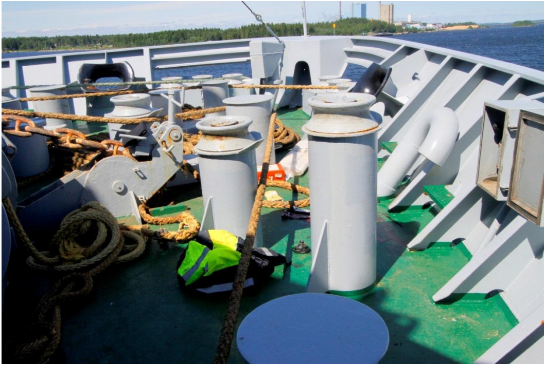
Fig. 3, Forecastle deck. To the right; the position of the chief officer when the accident occurred in the area of the platform at the remote control unit. To the left; the remaining of the parted spring line, piled up at its wind lass drum. (Photo from the Police)
