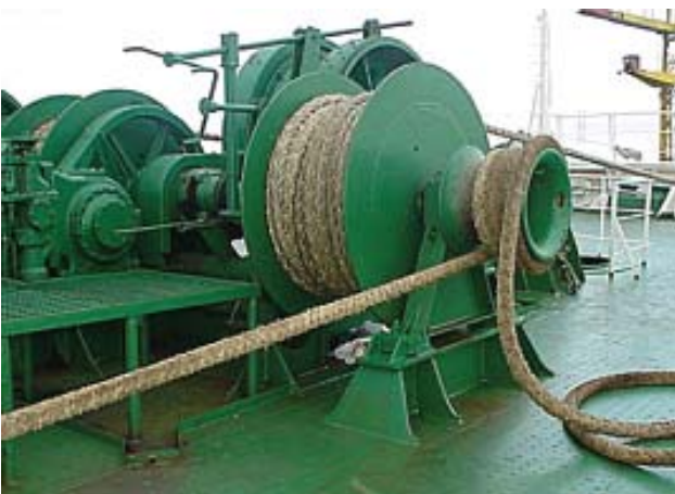
Well painted but poorly highlighted mooring station
