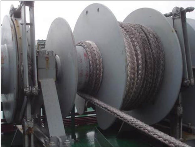
Correctly set up split drum
