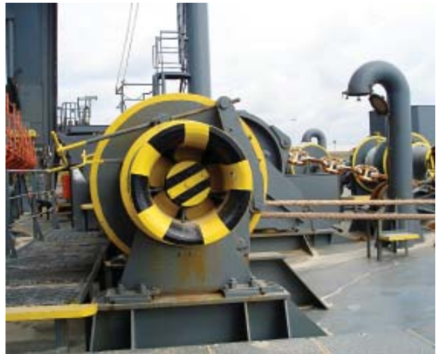
Mooring station with effective hazard markings
