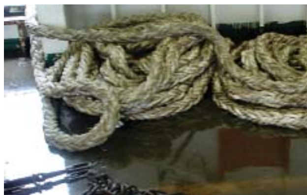
Ropes badly stored on wet deck
