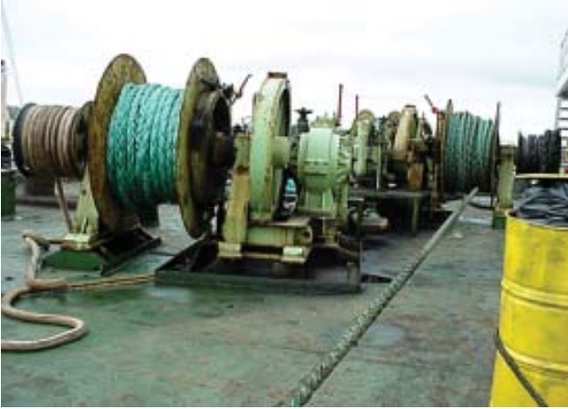
Mooring station with effective hazard markings
