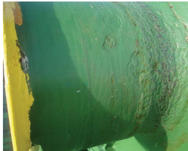
Build up of paint on the drum end
