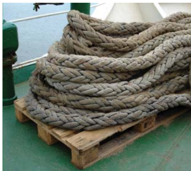
Ropes correctly stowed off deck
