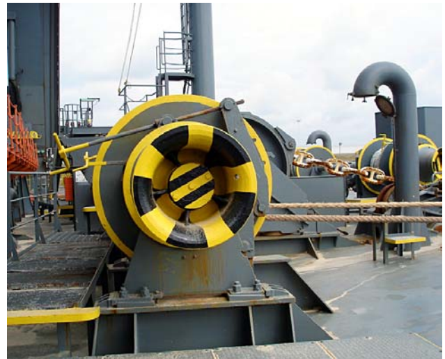
Mooring station with effective hazard markings
