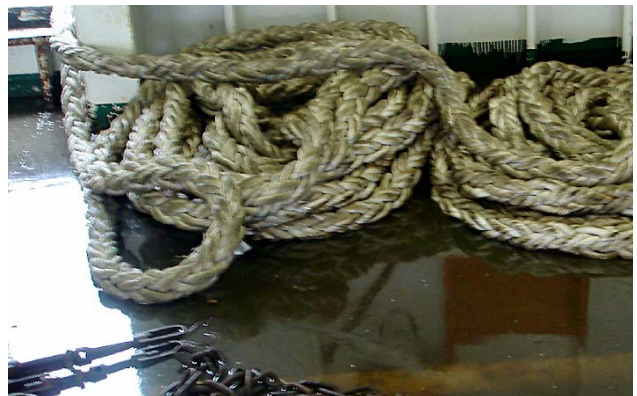
Ropes badly stored on wet deck
