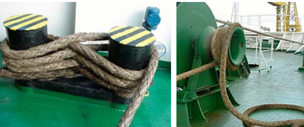
Once ropes have been hauled tight they should be secured to bitts as in the good example on the left
