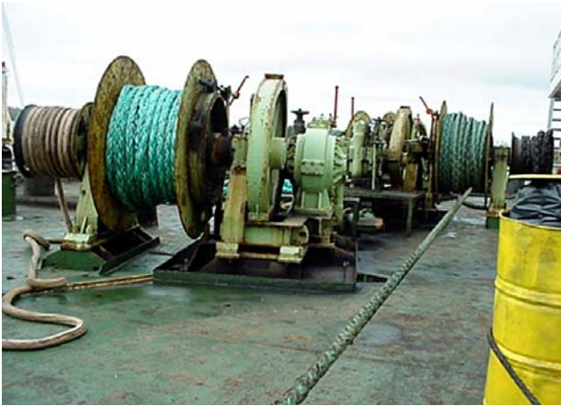
Mooring station with effective hazard markings
